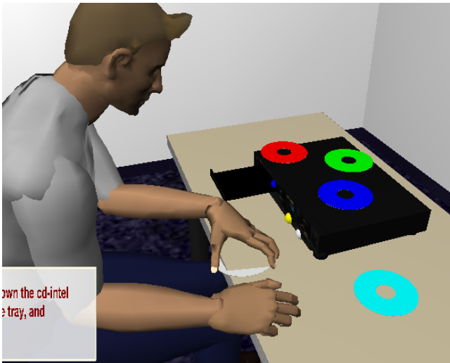
Figure 4: This figure shows a collision error. The hand with CD collides with the desk. The generic gestures combined with specific trajectory often result in such collisions.
